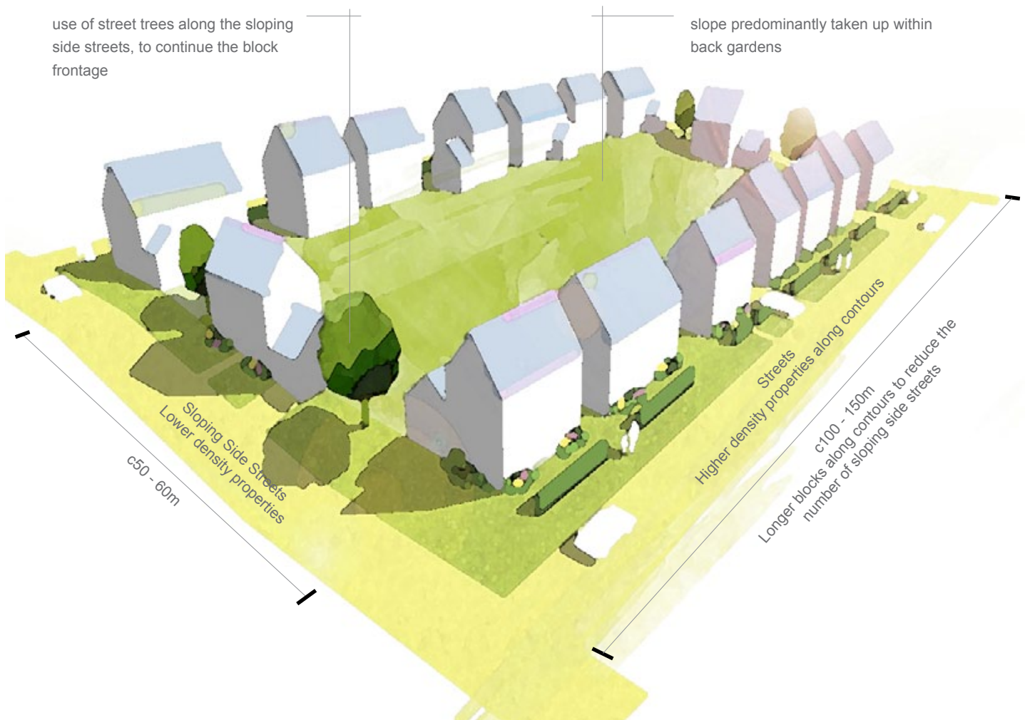
Typical closed block arrangement which could be adapted to respond to the underlying landform
